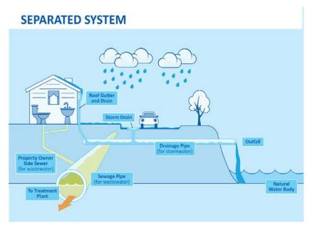
The picture shows the municipal separate storm sewer systems When you flush your toilet or run water down the drain, we have a separate sewage pipe for wastewater that goes to the treatment plant.
